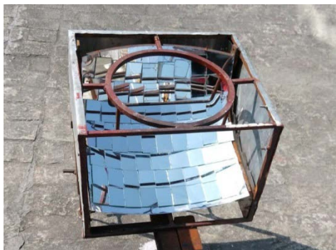
Fig. 4: Secondary reflector placed inside receiver
